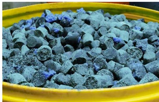
Figure 2: A barrel of copper nuggets with sulfate, ready to be recycled. Once the copper is mixed with sulfuric acid, it takes on a blue color.
