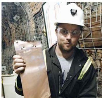
*Figure 3: Colter Dunagan holds a thin copper plate or anode, which is used to extract copper ions*
