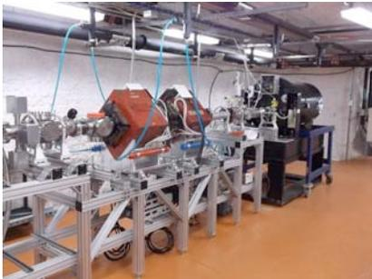
*Figure 1: Overview of the CASPAR accelerator with its tank closed and the first section of the beamline with a magnetic quadrupole doublet lens*
