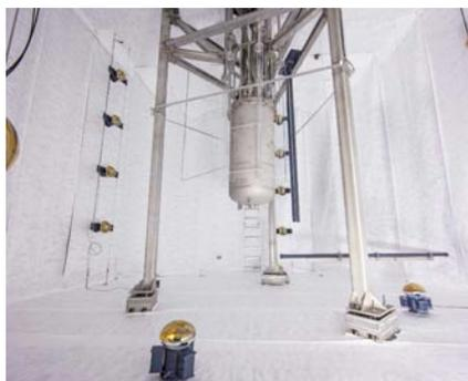
*Figure 7: LUX is housed in a 72,000-gallon tank 4850 feet underground*
