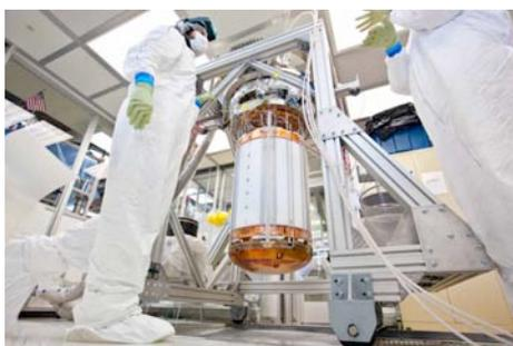
*Figure 6: 2013 photo of LUX researchers in a cleanroom at the Sanford Lab surface, working on the interior of the detector before it is inserted into its titanium cryostat*
