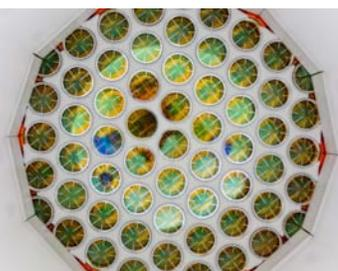
*Figure 7: Inside the Large Underground Xenon dark matter detector, arrays of photomultiplier tubes can detect a single photon of light*
